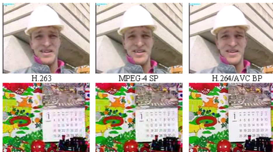
Figure 3. Comparison of picture quality for test sequences coded at 192 kbps with H.263, MPEG-4 SP and H.264/AVC BP
